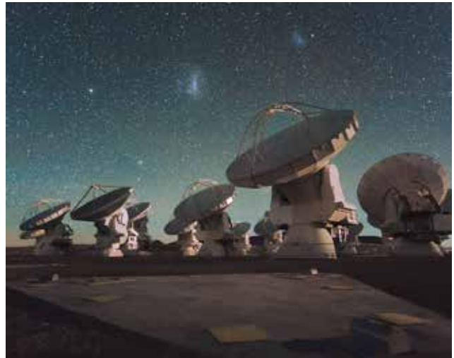
The ALMA (Atacama Large Millimeter Array) telescope, 5,000m high in the Andes. Data from 66 antennas are combined to provide remarkable resolution at millimetre radio wavelengths. Armagh has access through the UK membership of ESO.
