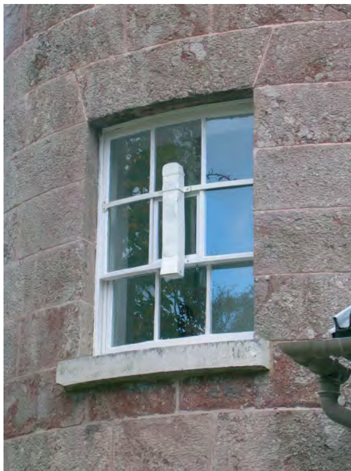
Figure 4. The light metal box at the north window of the East Tower at Armagh Observatory (photographed October 2004). This box housed the external thermometers used for Series I and the hygrometer used for Series III over the period from 1834 until the installation of the Stevenson screen in January 1884. This figure is available in colour online at www.interscience.wiley.com/ijoc
